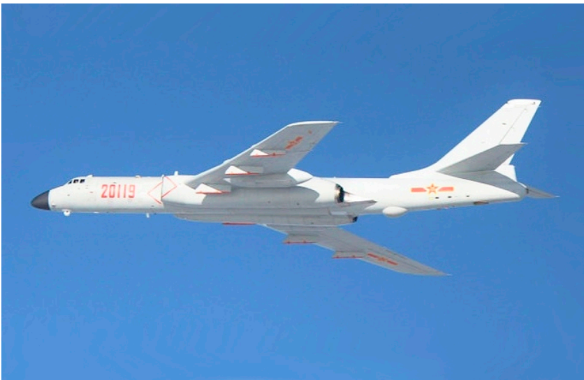
The Xian H-6K strategic bomber enjoys a much longer combat radius than its predecessor and is capable of carrying six missiles compared to two in previous versions. Image: Wikimedia commons.
